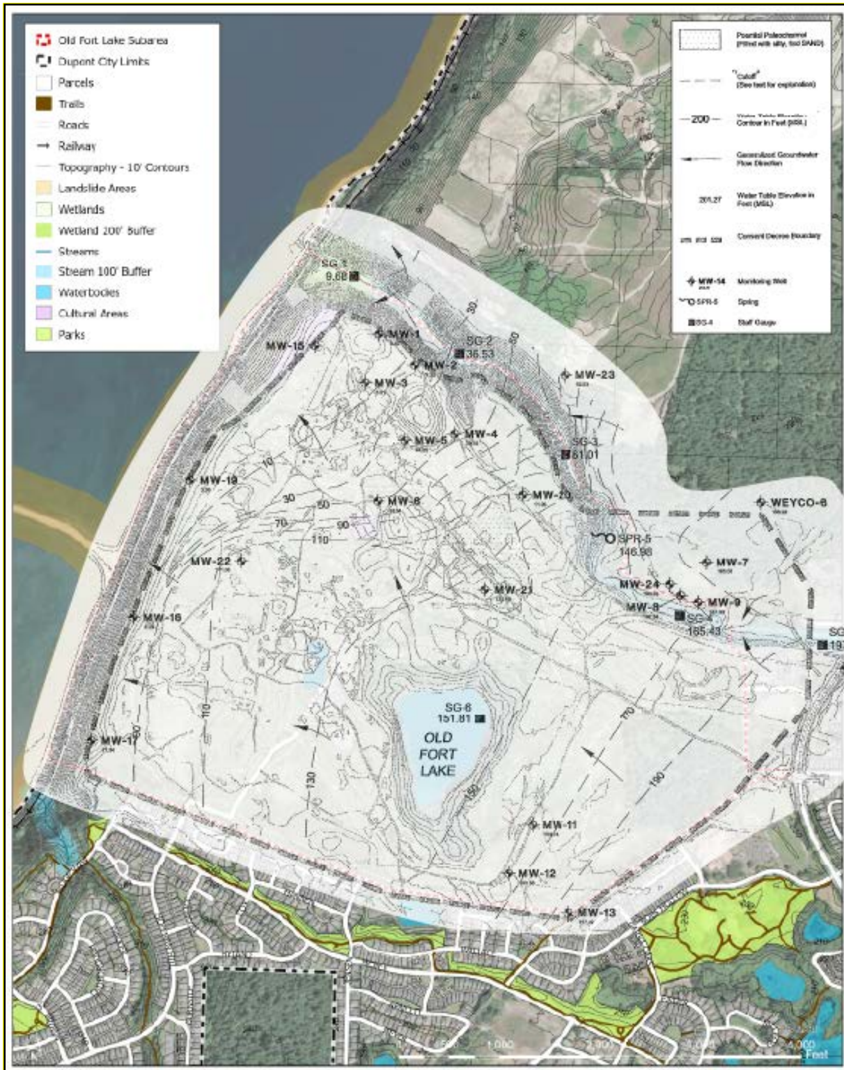
Figure 4-6 Groundwater Elevations Dry Season
