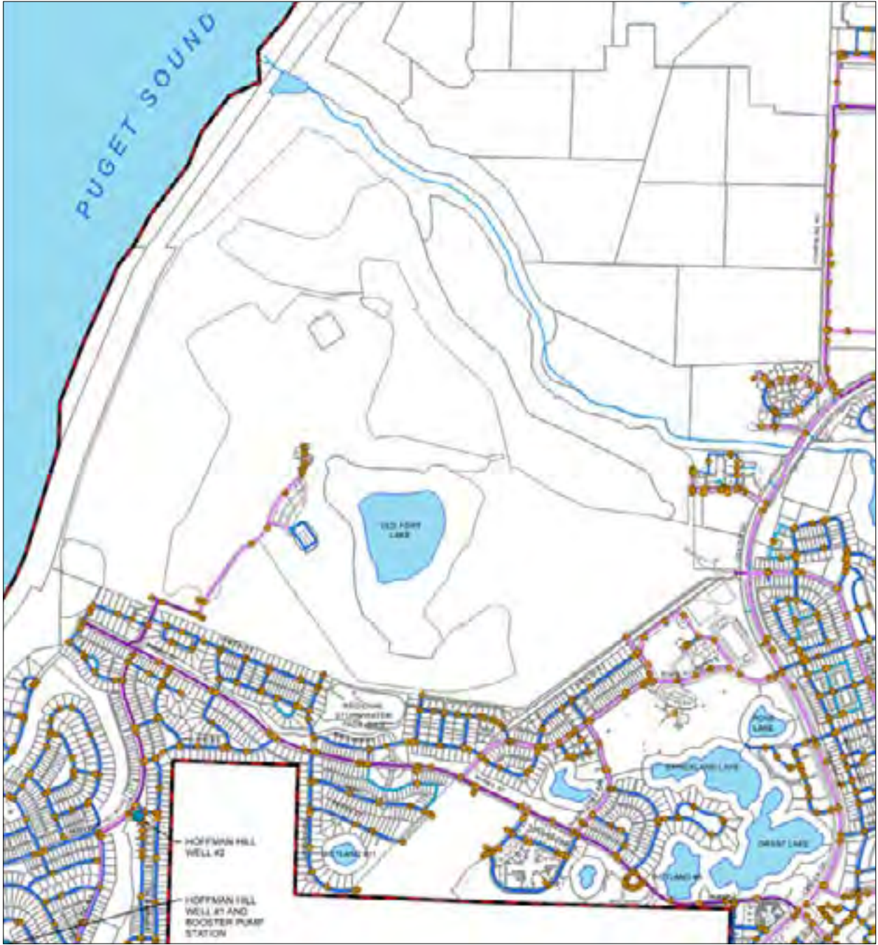
Figure 7-1. Water System Facilities Map
