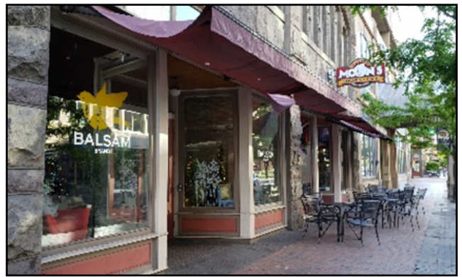
Figure 2 - Example of commercial building facade articulation using window patterns, weather protection, change in masonry texture and color.
